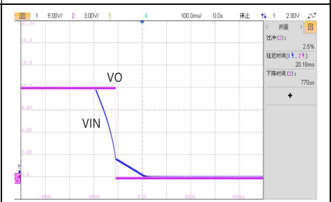
VIN=36V, 满载关机波形
