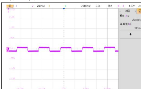
VIN=10.8V, 100%-10%-100%Io 动态波形
